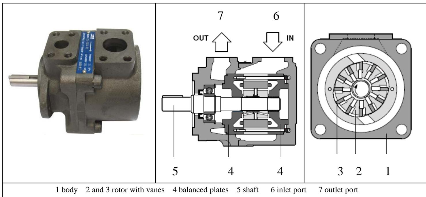
PFE are fixed displacement-twelve-vane pump, 2 and 3 cartridge design with integral hydraulic balancing 4 for high pressure operation and long service life with low noise level.
